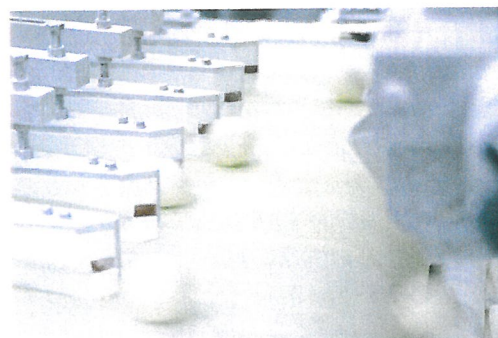
The dough divider divides 50,000 buns per hour. The dough pieces are brought into a uniform round shape by means of a moulding distance.
