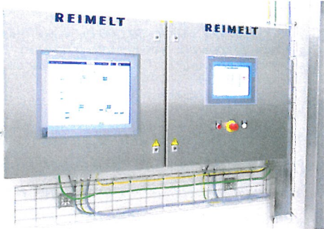
Control of the Codos system and the connected weighing. The complete complex can be shown in a graph.
