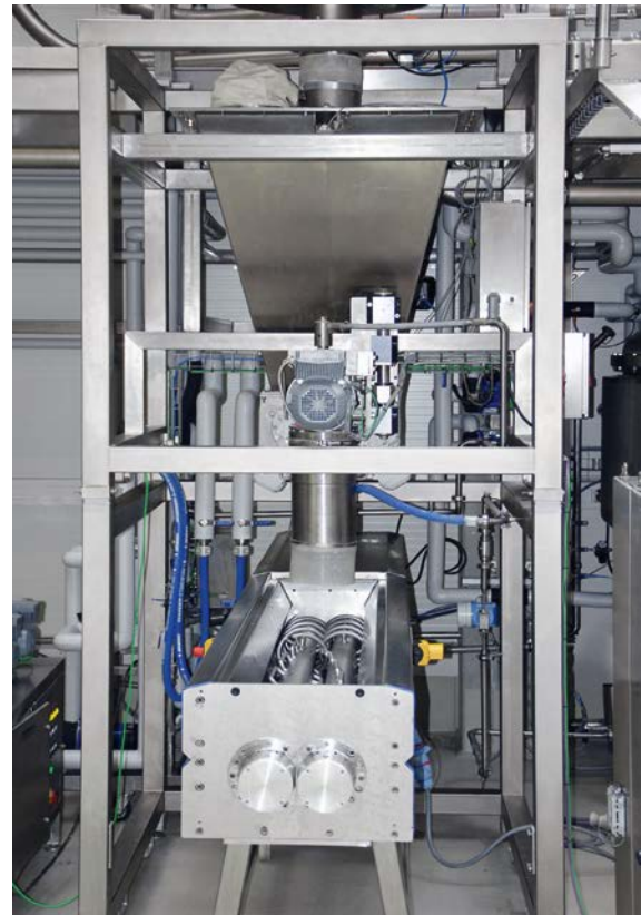
Gravimetric metering, DymoMix™ and Codos as well as pre-dough fermenters are available at the Zeppelin Technology Center in Rödermark for companies who want to carry out tests with their own raw materials.
