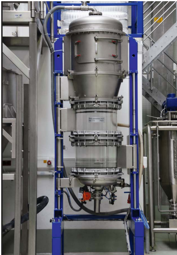
The Zeppelin Systems pneumatic mixer (homogenizing silo with fluidizing bed bottom) produces a homogeneous mixture without mechanics, friction or high friction.
