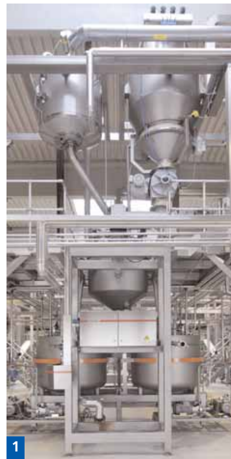
Picture 1: Preparation of sugar and glucose at a cooker for hard caramels
