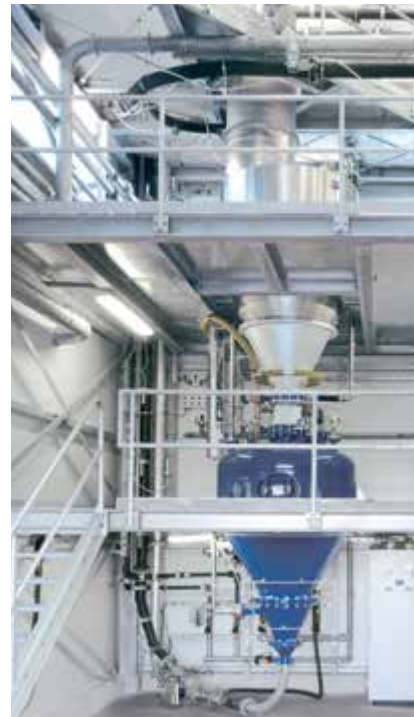
Discharge of powder from a pressure vessel.
