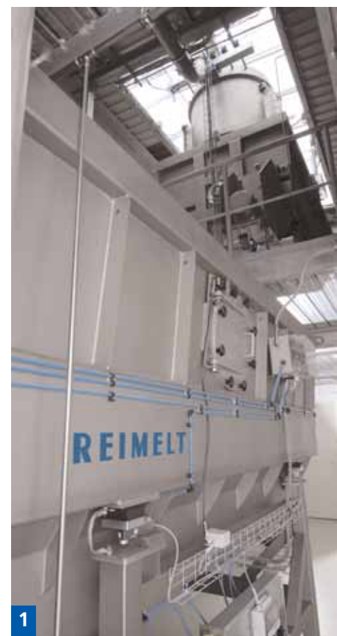
Picture 1: Agitator and recrystallization hoppers for powdered sugar
